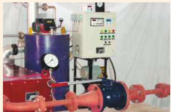
Microfinish research and development facilities include high temperature test loop to 480 °C (896 °F) at 15 bar pressure
